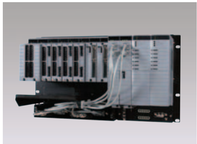
Figure 1 External View of FFCS CPU Node
